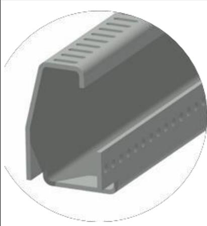
The unloading serves as an end stop for the transported material. In LIFO systems this profile is also used as loading profile. With the help of the locking bar the unloading profile is connected to the side profile. Even the unloading profile serves as loading of the fastening clips for roller tracks and guide rails.
